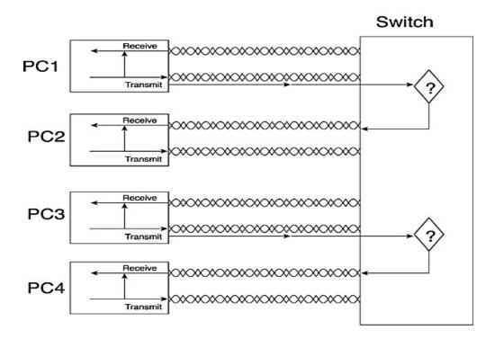
In above figure, both PC1 and PC3 are sending at the same time. The switch looks at the destination Ethernet address, and sends only the frame from PC1 to PC2 and the frame sent by PC3 to PC4. The big difference between the hub and the switch is that the switch interpreted the electrical signal as an Ethernet frame and processed the frame to make a decision. A hub simply repeats the electrical signal and makes no attempt to interpret the electrical signal (Layer 1) as a LAN frame (Layer 2).
