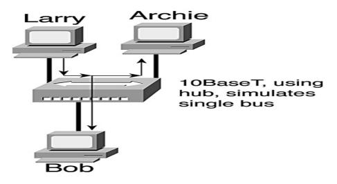
The concept of cabling each device to a central hub, with that hub creating the same electrical bus as in the older types of Ethernet, was a core fact of 10BaseT Ethernet. Because hubs continued the concept and physical reality of a single electrical path that is shared by all devices, we call this as *shared Ethernet:* All devices are sharing a single 10-Mbps bus.
